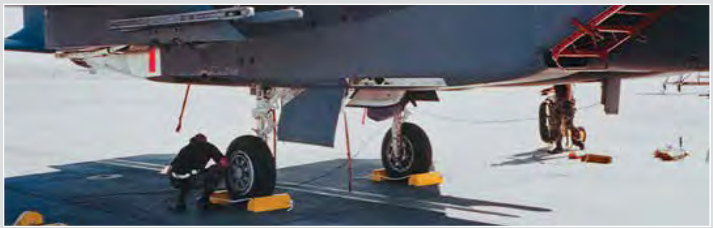
Monster AC6820-LR aviation chocks used on a McDonnell Douglas F-15 Eagle
